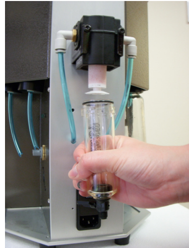
Figure 14b: Pull Down on Filter Bowl
