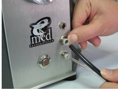
Figure 12: Removing Tubing from a Quick-Disconnect Fitting
